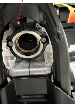
2.Install the spring retaining plate behind the guard. Install the M6x1.0x40  $\,$ . Using an 8 mm socket, tighten the bolts back into place. Make sure they are tightened securely, but don't over-tighten them.
