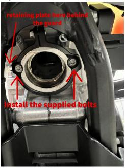
3.Using an 8 mm wrench finish tighten the M6x1.0x12
