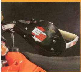
Enduro Engineering's new handguards are excellent. The new mounting system is U-shaped and makes room for cables and wiring.
