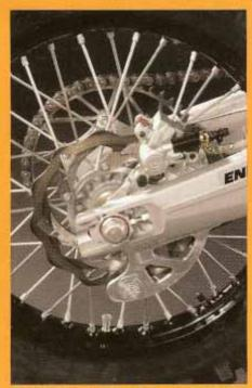
Out back we installed a Cooliger onto the rear brake line, and it helps cool the fluid. Enduro Engineering's shark fin is both tidy and tough.
