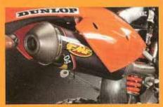
At 5 pounds 14 ounces, the full FMF Ti Q4 system shaved just about three pounds off of the tonnage. While bottom power was a shade softer than stock, mid to top was superb, and the D8 range is totally off-road legal.
