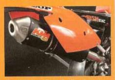
The KTM Hard Parts Q offered good power gains and kept the decibel level right on line with the production XC muffler. It's also just under one pound lighter than the KTM unit.
