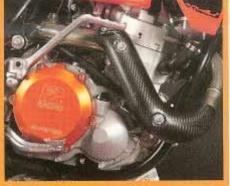
We have nothing but praise for the stock exhaust, once the inner tube is removed. Power is broad, the DB level is only slightly higher than stock, and it's strong. We did install an E-Line guard on the header, and this has saved our pants, which kept getting torched by the hot exhaust.
