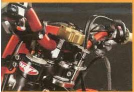
A BRP top clamp is rubber mounted and has a receptacle for a Scotts damper. The Scotts unit is inoffensive at slow speeds and performs miracles when the going gets nasty. The fork bleeders are SR Precision Parts and are small, out of the way, and perform flawlessty.
