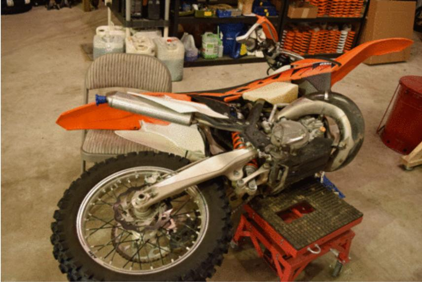
1. To prevent oil overflow, lay the bike on its LEFT SIDE (drive train facing the ground).
