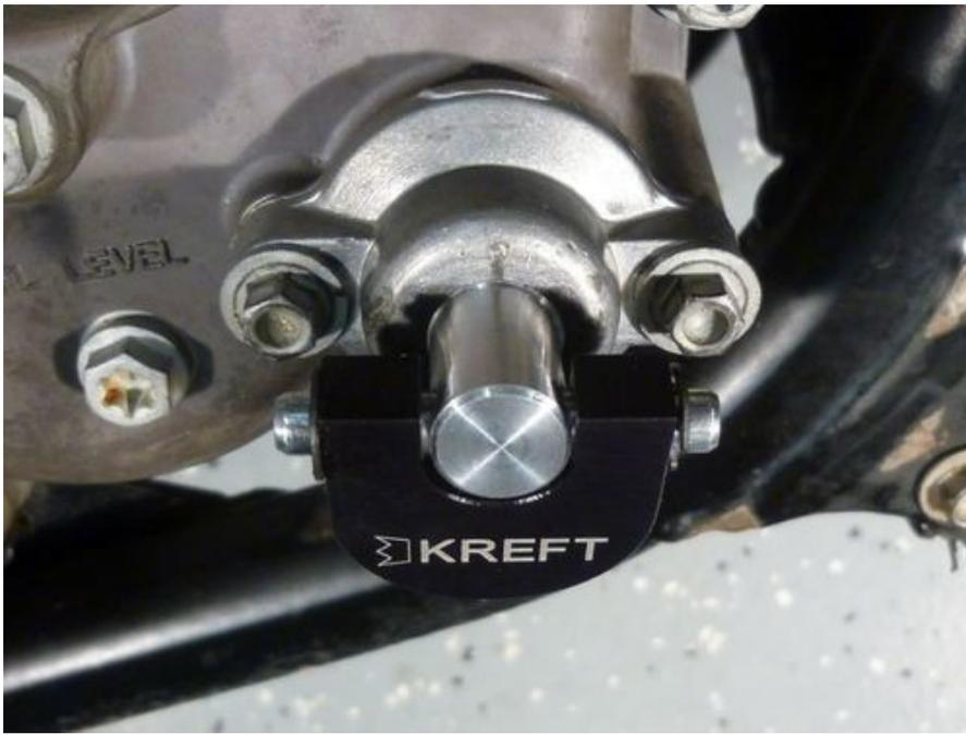
4. Your PowerDial spring guide comes with a new o-ring installed. Lubricate it with grease.
