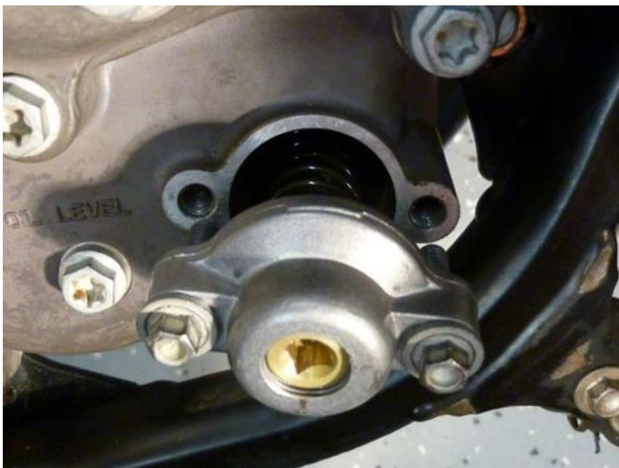
2. Unthread the 2 bolts on the power valve adjuster housing and remove the adjuster mechanism.
